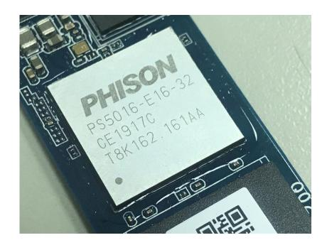
More faster PCle Gen4 x4 Phy: Dual-Core ARM base CPU, with built-in PCle PHY, fulfill high speed I/O Data read and write request.
