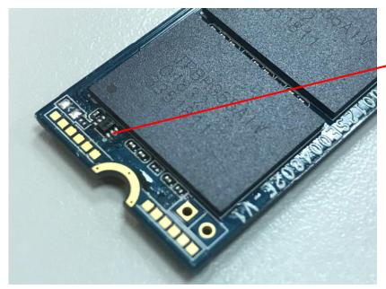
**External Thermal Sensor**: Location in the rear side of NAND to ensure more accurate temperature reading.
