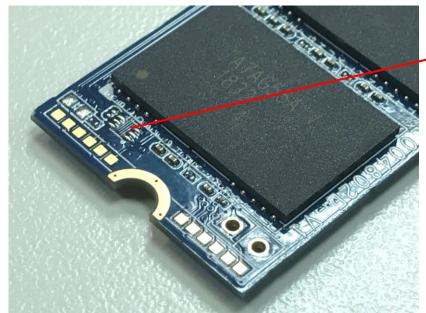
**W/O External Thermal Sensor**: Empty solder.
